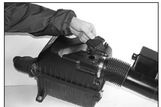
9. Loosen and remove the two screws that secure the mass-air sensor, then remove the mass air sensor.
