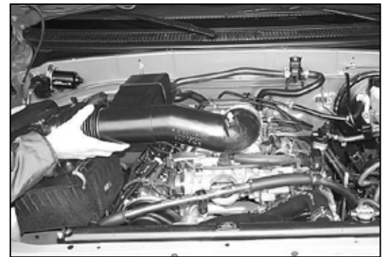
8. Remove the complete air intake system. NOTE: K&N Engineering, Inc., recommends that customers do not discard factory air intake.
