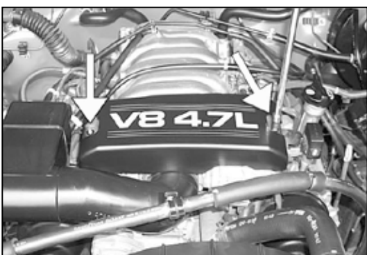
3. Loosen and remove the acorn nuts that secure the throttle body cover, then remove the cover.
